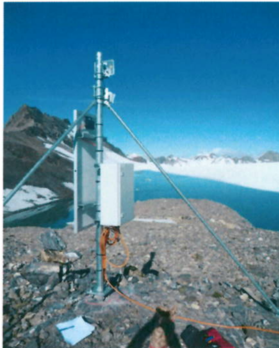
Figure 4: Example measuring station of GEOTEST/GEOPRAEVENT with autonomous power supply (solar panel, Plaine Morte glacier).
